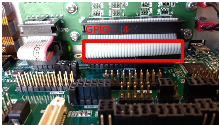
Figure 6.1. GR-CPCI-GR740 GPIO J4 connection.
