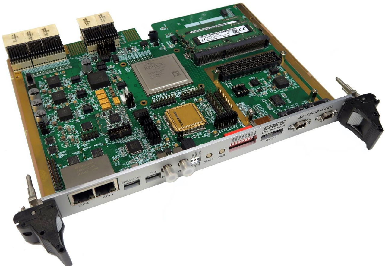
Figure 1 GR-CPCIS-XCKU Development Board
